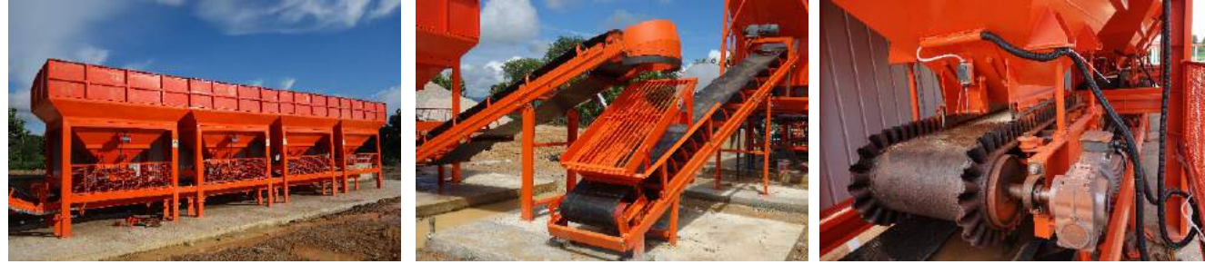
裙边带/ 缺料报警装置/ 电机减速机直连设计 Side wall type belt conveyor / Alarm sensor / Direct connection
